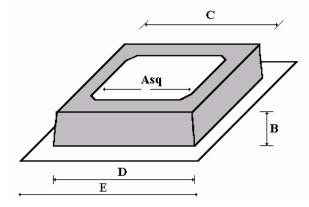
Designed specifically to provide load bearing support for roof mounted units, Grp support boxes may be installed in both pitched, or flat roof applications.
